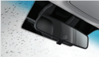
Rain sensor The rain sensor detects raindrops on the windshield and activates the wipers for clear visibility.
