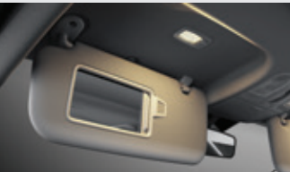
Sunvisor illumination lamps Bulb lamp over the vanity mirror on the driver-side sunvisor lights up to help you see yourself better in the mirror.
