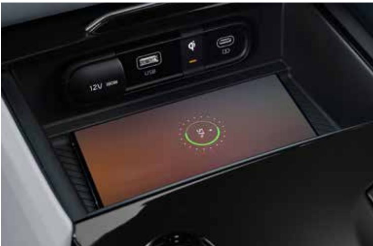
Wireless charging tray The charging pad in the dash, in front of the center console, lets you quickly charge compatible portable phones, wirelessly.
