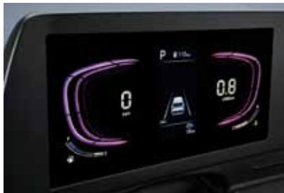
Supervision cluster (4.2-inch color TFT LCD)
