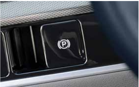
Electronic Parking Brake (EPB) Press the console EPB button when parking. EPB disengages in Drive or Reverse when you press the accelerator.
