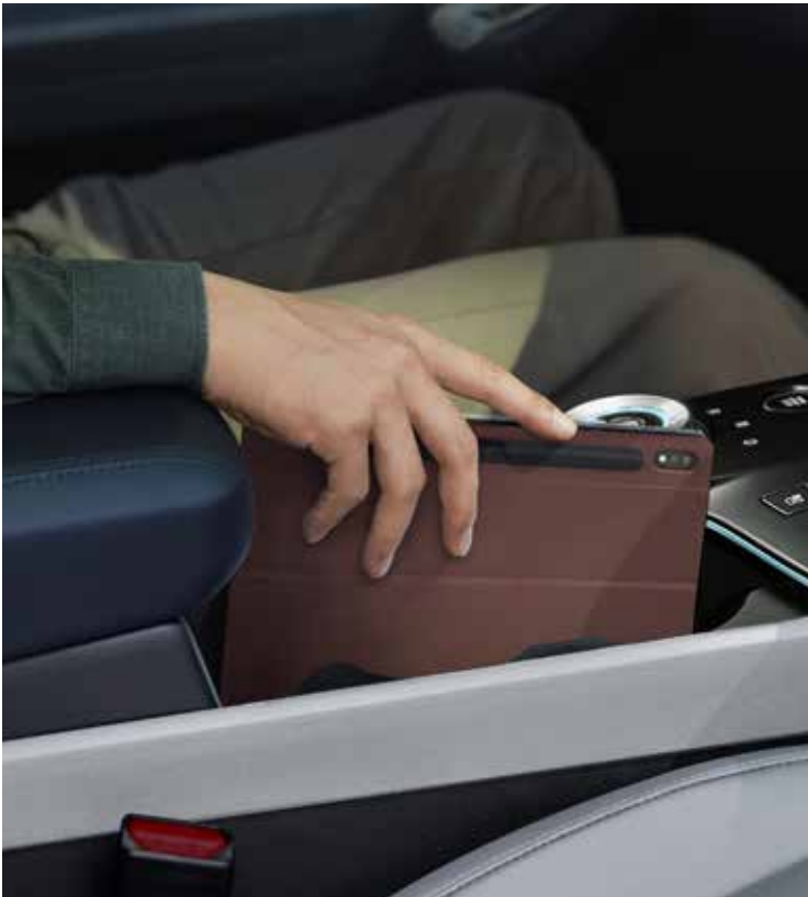
Variable cupholders & Multiple tray The center console cupholders disassemble when not in use, so tablets and other flat items can fit in the same space.
