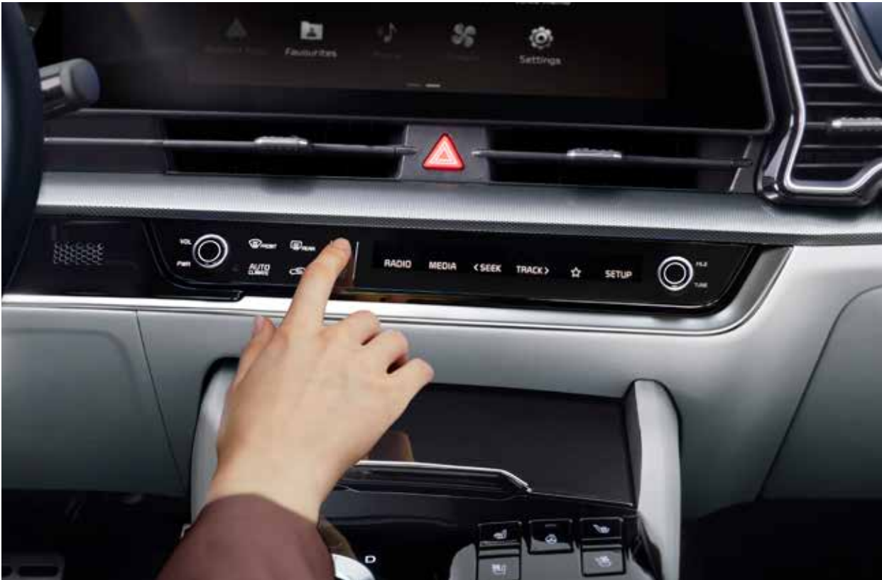
Infotainment/climate switchable controller Infotainment and climate functions share the same LCD softkey keyboard. Press the fan icon button to transform the controls on the right to climate. Press the arrow icon button to switch them to infotainment.
